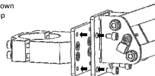
Depending on the operation style, D-type tool holder can be attached either horizontally or vertically.
