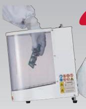
Powerful ionized air eliminates static electricity and blows away dust adhered on the workpiece. Pulse air function can also be selected to enhance the cleaning effect.
