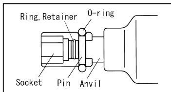
If it is not securely attached, the socket or bit may detach and fly off. Do not attach the socket or bit when the tool is idling.
