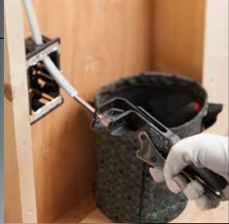
The 3200VA-1 is a solution for stripping strenuous cables such as VA cables which becomes soft and elongates during the summer or as eco-friendly PE cables, which hardness during winter months.
