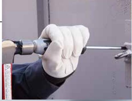
Our proprietary Tang-thru nut incorporates cam rotation mechanism, which turns the driving tip counter-clockwise by 12 degrees when the handle is hit with a hammer.
