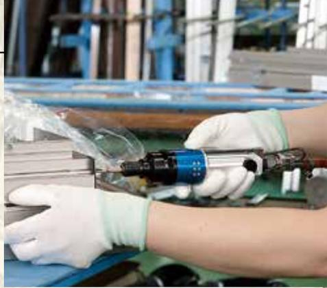
The Type A entry is designed to VESSEL's special insertion dimensions, developed when we first started manufacturing air drivers. The majority of electric drivers on the market can be used with our ubiquitous Type A bits.
