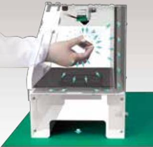
Static electricity elimination and dust removal in a hood. Dust adhered by static electricity is neutralized in the ionized hood and then removed by powerful automatic air blow.
