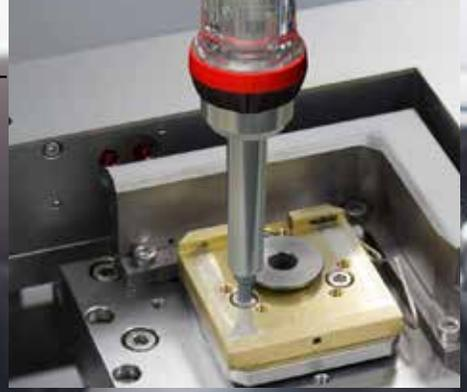
This functionally enhanced screwdriver enables screw tightening by simple repeated wrist movements.
