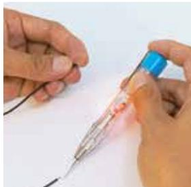
Continuity check of a wiring circuit
