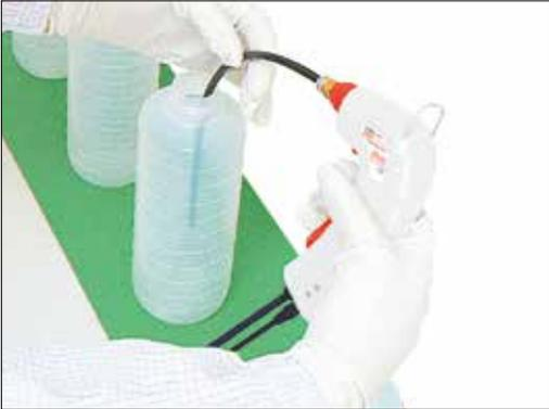
Static electricity removal in a bottle
