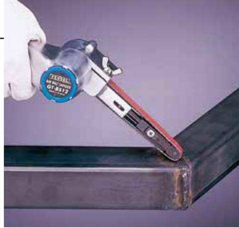
The center of the arm becomes the center of gravity. This belt has been designed in an offset position so that it becomes aligned with the center of the arm when the unit is taken up. This slight difference in balance makes a big difference in reducing fatigue. A major ergonomic achievement.
