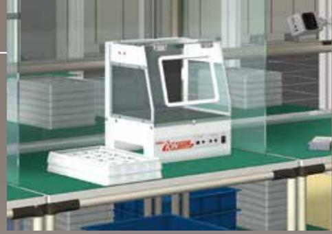
With the Ion parts cleaner applying a unique dust capturing method with an adhesive gel sheet, an installation space for a dust collector or a dust is no longer needed. This gel sheet can be repeatedly used after cleaning off dust.
