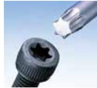
TORX has 6-lobe shaped curves. Compared to hexagonal shape driver, TORX has higher drive effectiveness and transfers torque smoothly and accurately while eliminating "CAM-OUT".
