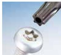
Added function of "Never Touch Screw" a post in the middle of the recess for maximum security eliminates regular TORX drive or any other flat screwdrivers for safety. Tamper proof screws are mostly used at communication equipment and computers so as not to abuse the screwing/unscrewing due to its design and control of function. Keep off unscrewing unless otherwise maintenance serving practiced.
