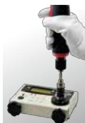
Either the Peak Hold measurement mode suitable for measuring electric screwdrivers, or the Peak Down Hold measurement mode suitable for manual tools can be selected.
