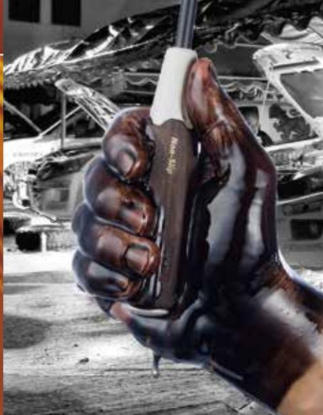
Maintenance of cars, motorbikes and machines always involves oils. Wood-compo screwdriver's coarse wood powder on the grip surface stops the oil flow against the tightening torque, producing an outstanding non-slip grip effect.
