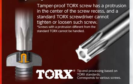
**TORX**® Tip-end processing based on TORX standards. Corresponds to various screws.
