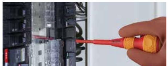
For prevention of electric shock or short-circuit during electric works for power equipment, telecommunication devices, electric vehicles, solar power stations, and so on.
