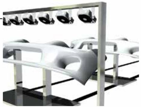
This type adopts a piezoelectric transformer that is safe and superior in ion generation. In addition, VESSEL's specific capacitive coupling method in which a discharge needle is sandwiched with resin and stainless disc, enables unmatched good ion balance.
