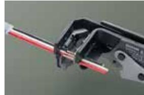
Wire strippers dedicated for VA cables and eco-friendly PE cables (VVF/EM-EEF)
