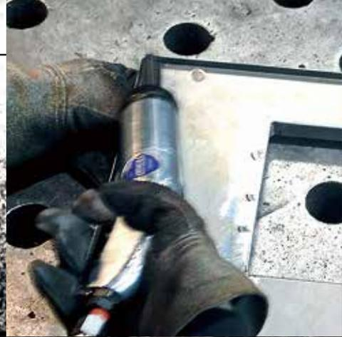
The barycenter is at the front side, alleviating the strain on your wrist. Effortless operation is possible by just pressing the needles on welding spatters, slugs, etc. The impact does not catch your hand so the needles do not spread out as much, making it easier to work.
