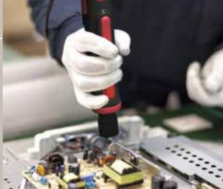
The ergonomic design that reduces the burden on the worker during consecutive assembly and/or fastening work.
