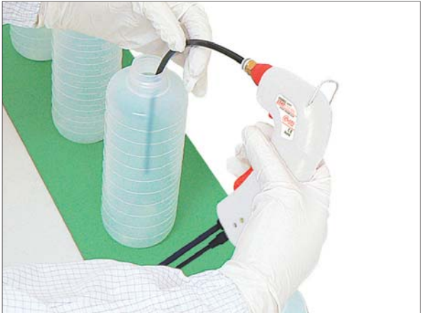
Static electricity removal in a bottle
